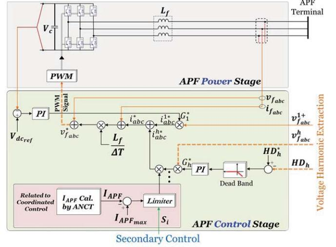
Fig. 6. APF power stage and control structure.
