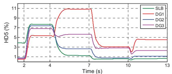
Fig. 13. 5<sup>th</sup> Voltage harmonic distortion (Scenario 1).
