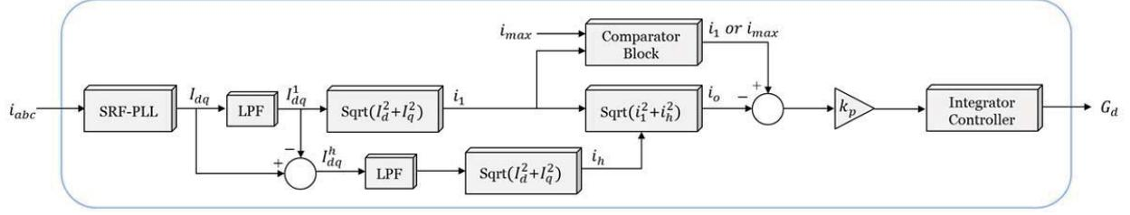
Fig. 9. Block diagram of inverter nominal power constraint.
