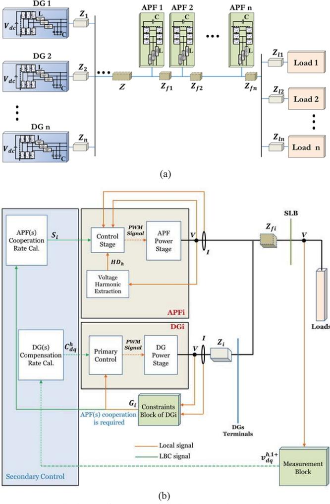
Fig. 1. General scheme of: (a) microgrid, (b) proposed control.
