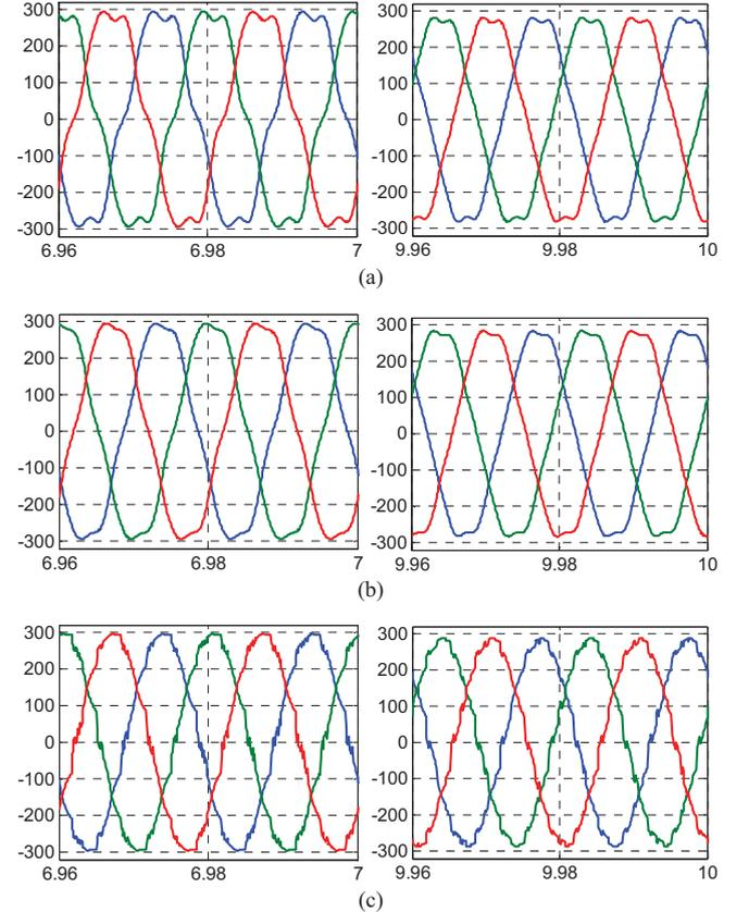
Fig. 16. Voltage waveform (Scenario 2): (a) DG<sub>1</sub>, (b) DG<sub>2</sub>, (c) SLB.
