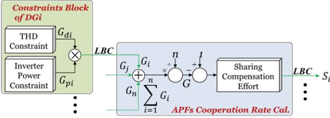
Fig. 7. Block diagram of coordination process.
