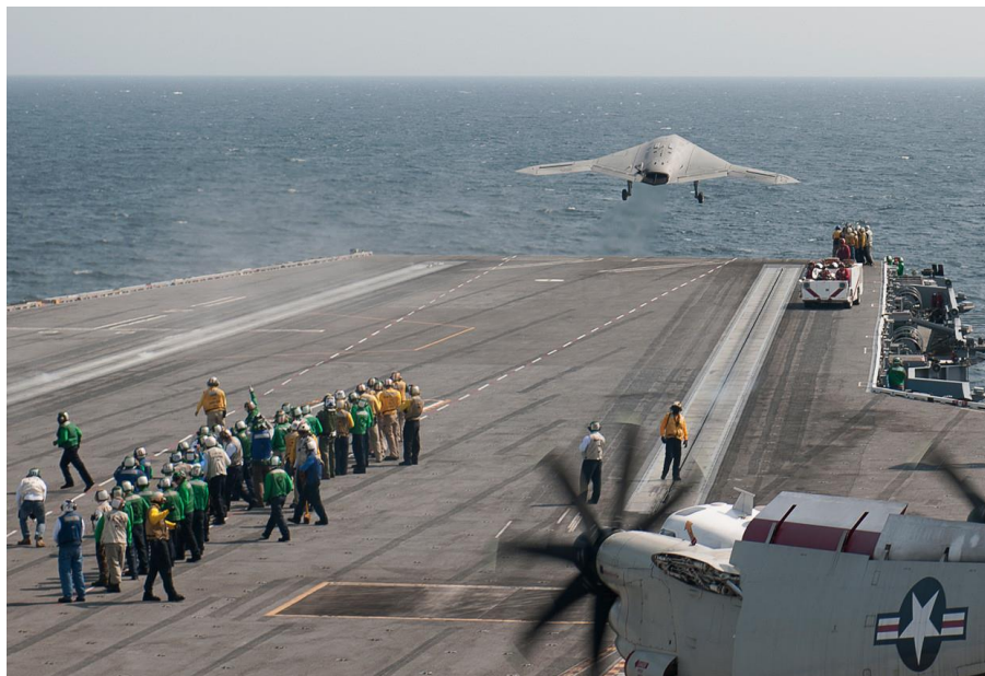
Figure 1: X-47B UCAS armed drone completes takeoff, refueling and landing completely unassisted by humans.
