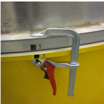
Figure 41: Clamp for tightening the aluminium frames to the sand box edge.
