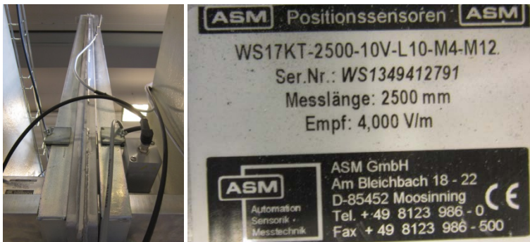
Figure 24: Displacement transducer for hydraulic cylinder 1.
