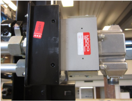
Figure 27: Displacement transducer for Hydraulic cylinder 2.
