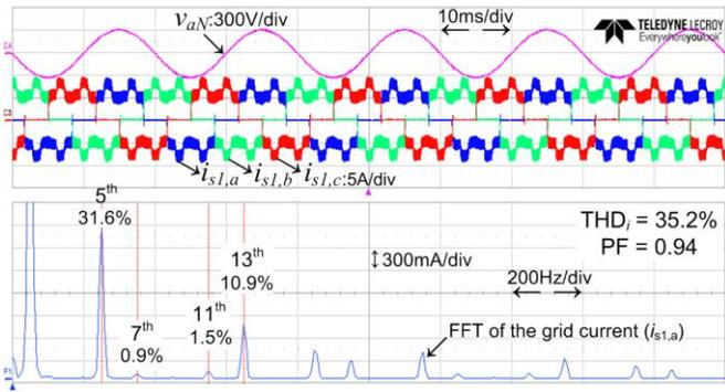
Fig. 9. Experimental results (phase a) of a rectifier unit with the proposed compensated predictive current modulation control at  $P_o \approx 3$  kW, targeting at eliminating 7<sup>th</sup> and 11<sup>th</sup> harmonic orders: grid phase voltage  $v_{aN}$  [300 V/div], diode rectifier input currents  $i_{s1,abc}$  [5A/div] and Fast Fourier Transform (FFT) analysis of the diode rectifier input current  $i_{s1,a}$  [300 mA/div].
