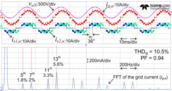
Fig. 10. Experimental results (phase a) of the multi-rectifier system with the proposed compensated predictive current modulation control **targeting at minimizing 5<sup>th</sup>, 7<sup>th</sup> and 11<sup>th</sup> harmonic orders**: grid current  $i_{g,a}$  [10 A/div], grid phase voltage  $v_{aN}$  [200 V/div], diode rectifier input current  $i_{s1,a}$  [10A/div], SCR unit input current  $i_{s2,a}$  [10 A/div], and Fast Fourier Transform (FFT) analysis of the grid current [200 mA/div].
