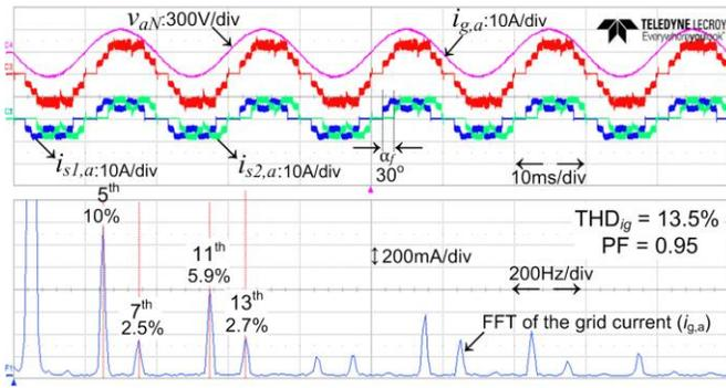
Fig. 13. Experimental results (phase a) of the multi-drive system with the proposed compensated predictive current modulation control **targeting at a minimized THD<sub>ig</sub> and improved PF**: grid current  $i_g$  [10 A/div], grid phase voltage  $v_{aN}$  [200 V/div], diode rectifier input current  $i_{sa1}$  [10 A/div], SCR unit input current  $i_{sa2}$  [10 A/div], and Fast Fourier Transform (FFT) analysis of the grid current [200 mA/div].
