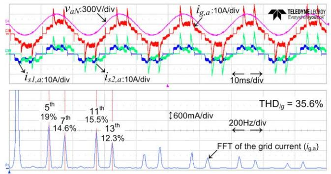
Fig. 11. Experimental results **without including the compensation** in the predictive controller for the case targeting at minimizing 5<sup>th</sup>, 7<sup>th</sup> and 11<sup>th</sup> harmonic orders: grid current  $i_g$  [10 A/div], grid phase voltage  $v_{aN}$  [300 V/div], diode rectifier input current  $i_{s1,a}$  [10 A/div], SCR unit input current  $i_{s2,a}$  [5 A/div], and Fast Fourier Transform (FFT) analysis of the grid current [600 mA/div].
