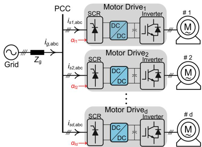
Fig. 1. Schematic of a multi-drive system applying a pulse pattern current modulation strategy at DC link employing a DC-DC converter.
