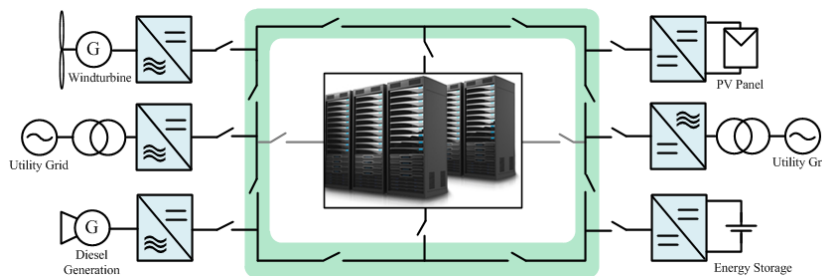
Fig.3 Ring-bus based DC microgrid
