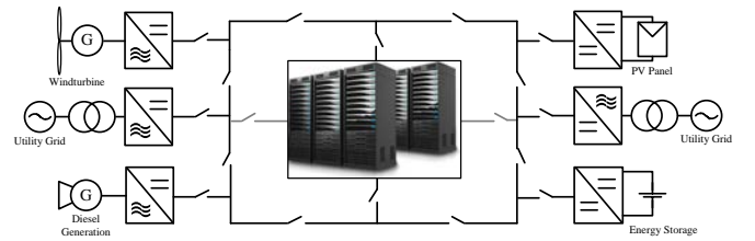
Fig. 2. Ring-bus based DC microgrid feeding critical load.
