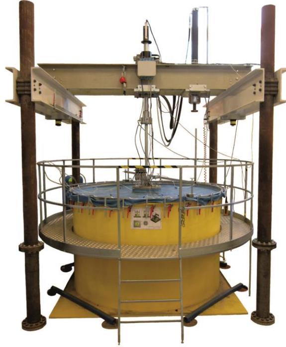
Fig. 2. Setup for a test with applied suction.
