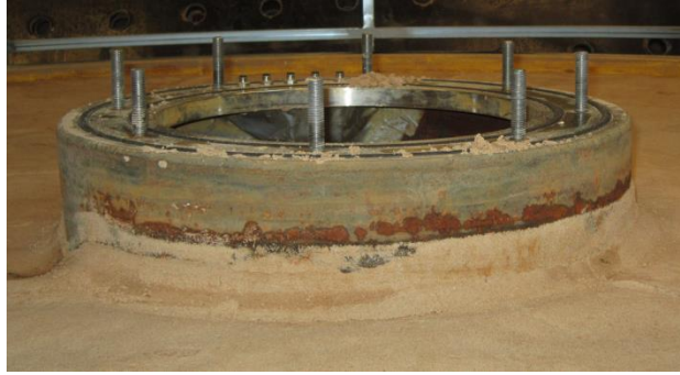
Fig. 4. After tests with applied suction, sand in the interface is stuck to the pile.
