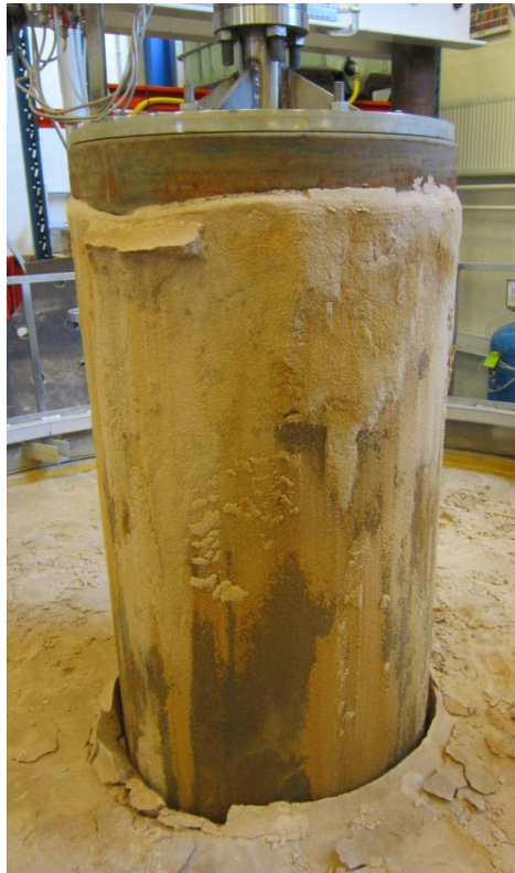
Fig. 5. Uninstallation of the pile after a test with applied suction. Sand is not resaturated before uninstillation, and some sand is stuck to the upper one third of the pile.
