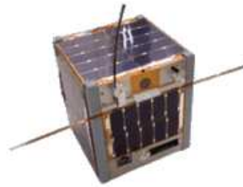
Figure 2. The XI-IV Cubesat to be deployed from SSETI-Express
