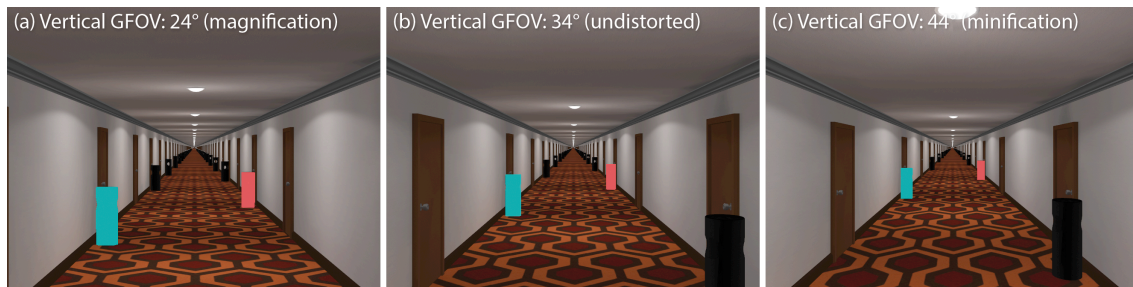
Figure 6. The three vertical GFOV used in S4. To make the distortion more easily apparent two virtual objects are highlighted in blue and red.
