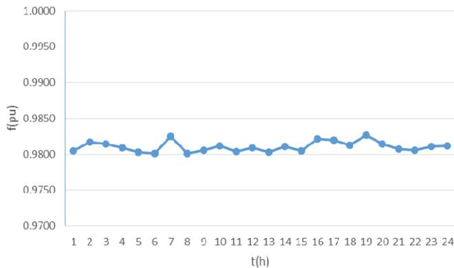
Fig. 8. The frequency of system in 24 hours after performing optimized power flow
