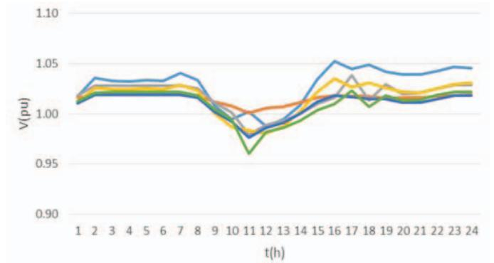
Fig. 9. The voltage of 6-bus of the system in 24 hours after performing optimized power flow
