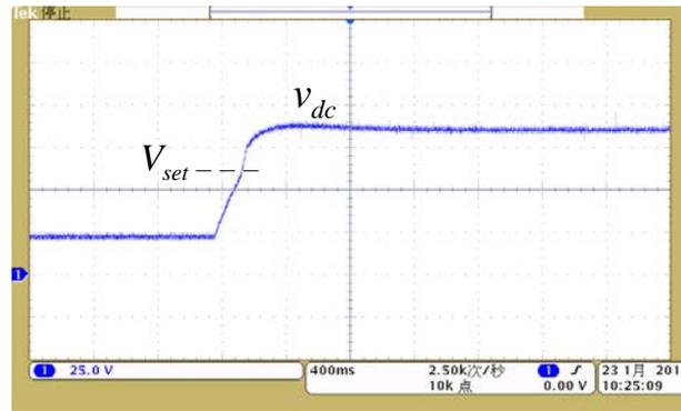
Figure 9. Start-up process of dc-link voltage
