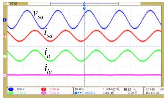
Figure 10. Harmonic compensation results with nonlinear load disconnected
