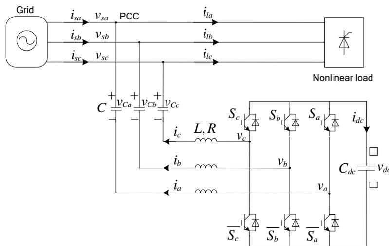
Figure 1. Topology of parallel hybrid active power filter
