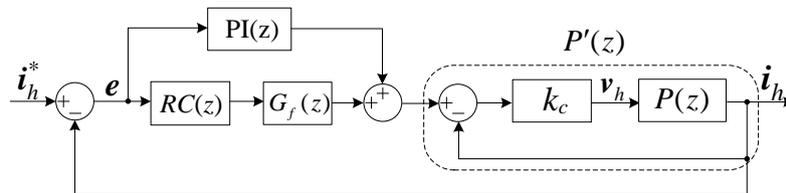
Figure 6. Block diagram of harmonic current tracking control
