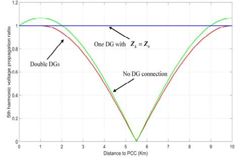
Fig.14. 5<sup>th</sup> harmonic mitigation along the feeder
