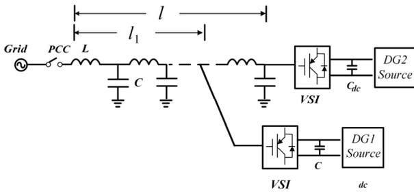
Fig. 8. Diagram of two DG's installation points
