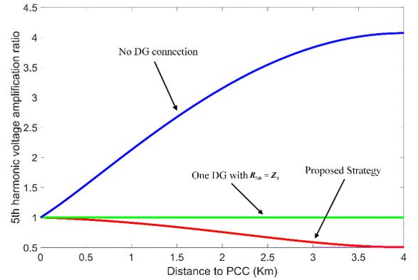
Fig. 10. 5<sup>th</sup> harmonic mitigation along the feeder
