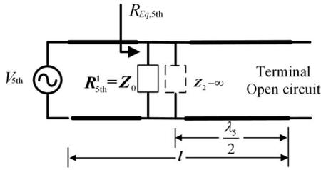
(a) 5<sup>th</sup> harmonic equivalent model of feeder
