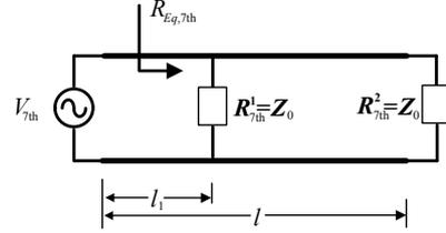
(b) 7<sup>th</sup> harmonic equivalent model of feeder
