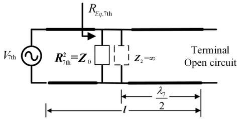
(b) 7<sup>th</sup> harmonic equivalent model of feeder
