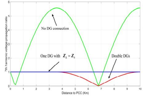
Fig.15. 7<sup>th</sup> harmonic mitigation along the feeder
