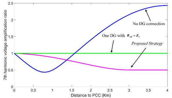
Fig. 11. 7<sup>th</sup> harmonic mitigation along the feeder
