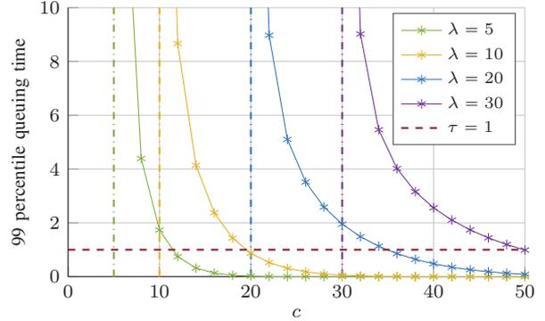
Fig. 5. The 99-percentile queuing delay vs. the number of servers for different arrival rates, where  $\lambda = \lambda_1 = \lambda_2$ . The dashed horizontal line indicates  $\tau = 1$ , and the dash-dotted lines show the asymptotes.
