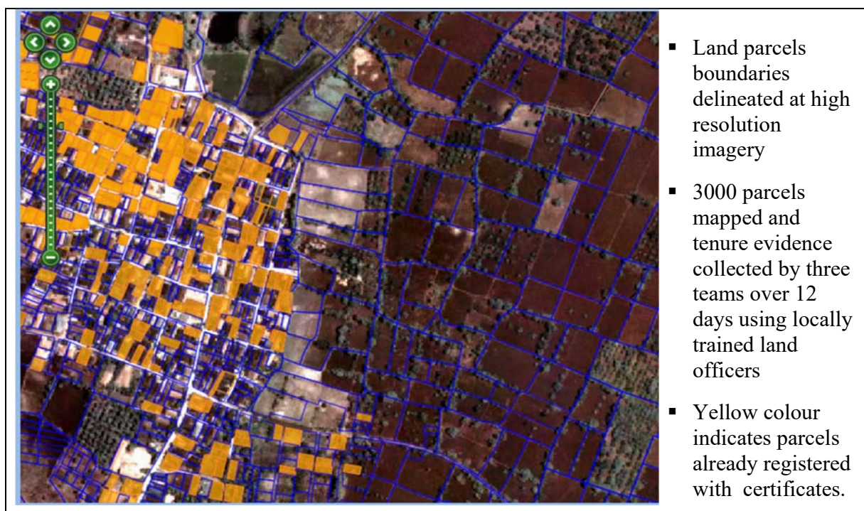
Figure 6. Example of demarcation of land parcels using high resolution imagery. Wotan Village, Gresik District, East Java Province, Indonesia (Source: Gresik District Land Office, East Java province).
