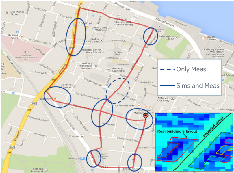
Fig. A.2: Handovers location and zoom of an area where a building's footprint crosses a street due to the 5x5 m map resolution.
