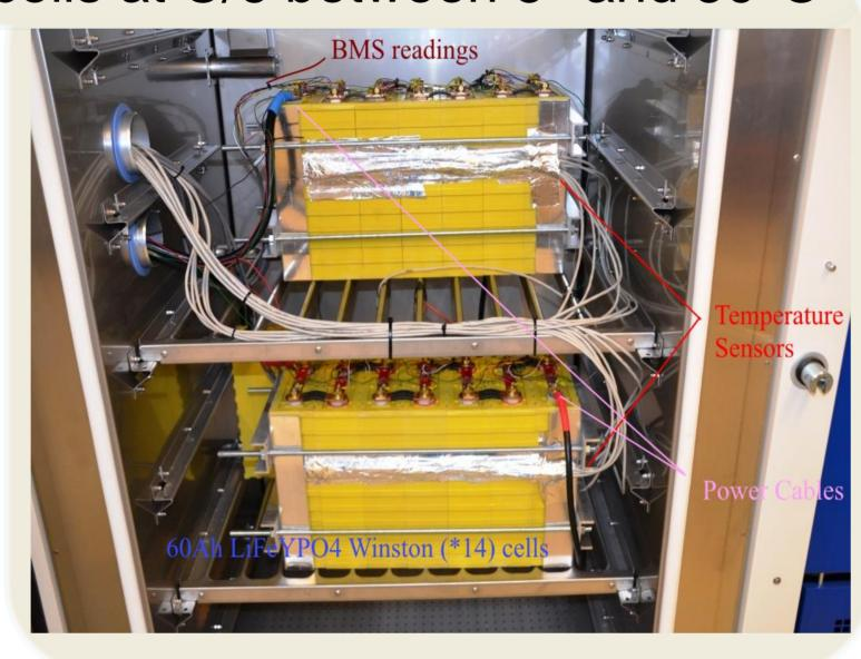
14\*CALB 60Ah LiFePo4 cells at C/5 and C/10 charge current rate
