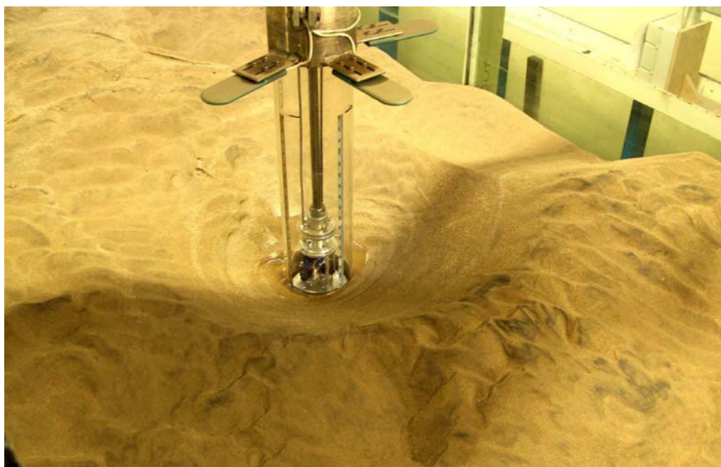
Figure 5-6: A live-bed scour hole.
