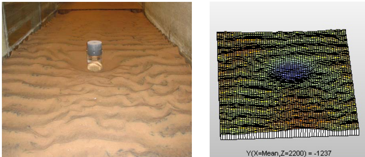
Figure 7. Picture and profiler measurement showing scour hole after 1500 waves. Test 1.5.
