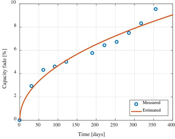
Fig. 10. Measured and estimated capacity fade of the NMC-based Li-ion cells.
