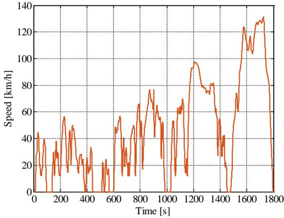
Fig. 3. WLTC driving cycle for a Class 3 vehicle.
