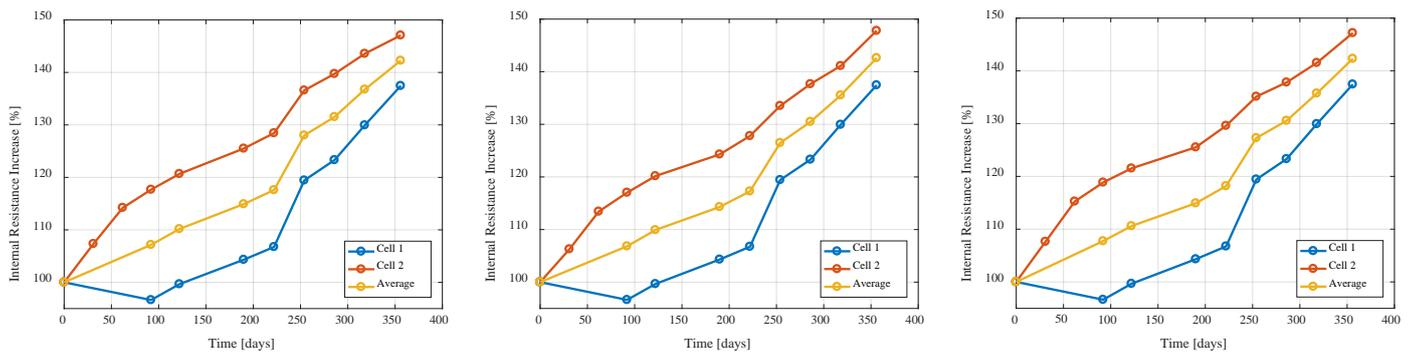
Fig. 13. Internal resistance increase measured at 20% SOC (left), 50% SOC (centre), and 80% SOC (right) for a 1.5 C-rate discharging pulse.
