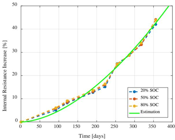
Fig. 14. Measured internal resistance increase at different SOC levels and estimated resistance increase; internal resistance measured during a charging current pulse.
