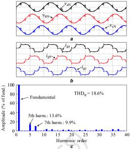
**Fig. 5** Simulation results of the multiple parallel ASD system consisting of four SCR-fed drive units with linearly designed firing angles  $(0^{\circ} \le a_f \le 30^{\circ})$ : (a) grid phase voltages  $v_{abc,N}$  [400 V/div], (b) total grid currents [40 A/div], time [10 ms/div], and (c) the Fast Fourier Transform (FFT) of the phase-a grid current  $i_{ga}$ .
