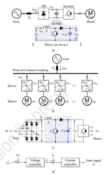
Fig. 1 Examples of the DR-fed drive systems: (a) single-drive unit with a boost dc-dc converter in the dc-link, (b) multi-drive systems (n drive units), (c) hardware schematic of an SCR-fed three-phase drive system with a boost converter in the dc-link, and (d) control structure of the boost dc-link stage.
