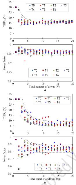
**Fig. 2** Performance of a multi-drive system considering various number of drives under different loading conditions with linearly dispatched firing angles (Top: THD level of the total current at PCC, i.e., the grid current; Bottom: resultant power factor): (a)  $0^{\circ} \le \alpha_f \le 30^{\circ}$  and (b)  $0^{\circ} \le \alpha_f \le 60^{\circ}$ . If there is no phase-shifting (all DR-fed drives), a THD of 31% and a power factor of 0.96 will be obtained.
