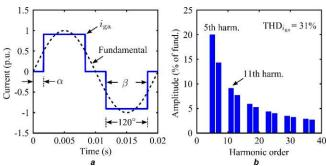
**Fig. 2** Harmonic characteristics of the phase-a current drawn by a SCR drive system: **(a)** ideal current waveform  $(\alpha = \alpha_f + 30^\circ \text{ and } \alpha_f = 0, \beta = 120^\circ)$  and **(b)** harmonic distribution.
