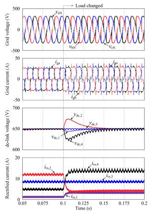
**Fig. 7** Transient performance of the multi-drive system consisting of four SCR-fed drive units with the deliberately dispatched firing angles, i.e.,  $a_f = [0, 10^\circ, 20^\circ, 30^\circ]$ , where the subscripts (i.e., 1, 2, 3, and 4) represent the drive number.
