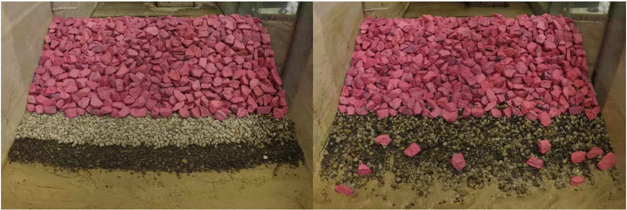
Figure 19: The front of the breakwater (C2) is shown on both pictures. Left shows before Test 12 and right shows after Test 14.
