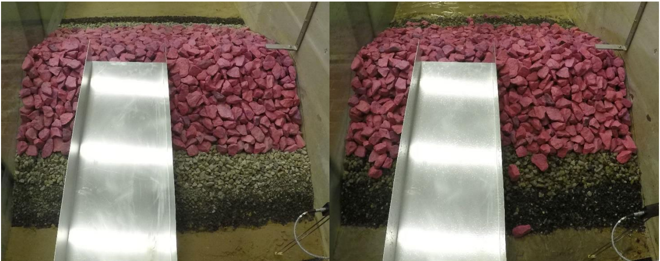
Figure 17: The rear of the breakwater (C1) is shown on both pictures. Left shows before Test 1 and right shows after Test 6.
