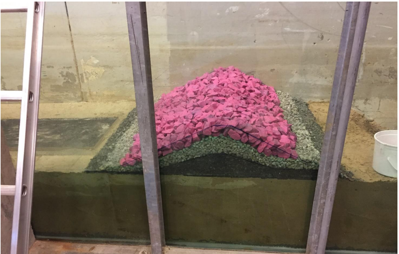
Figure 7: Breakwater with armour layer for cross-section C1.
