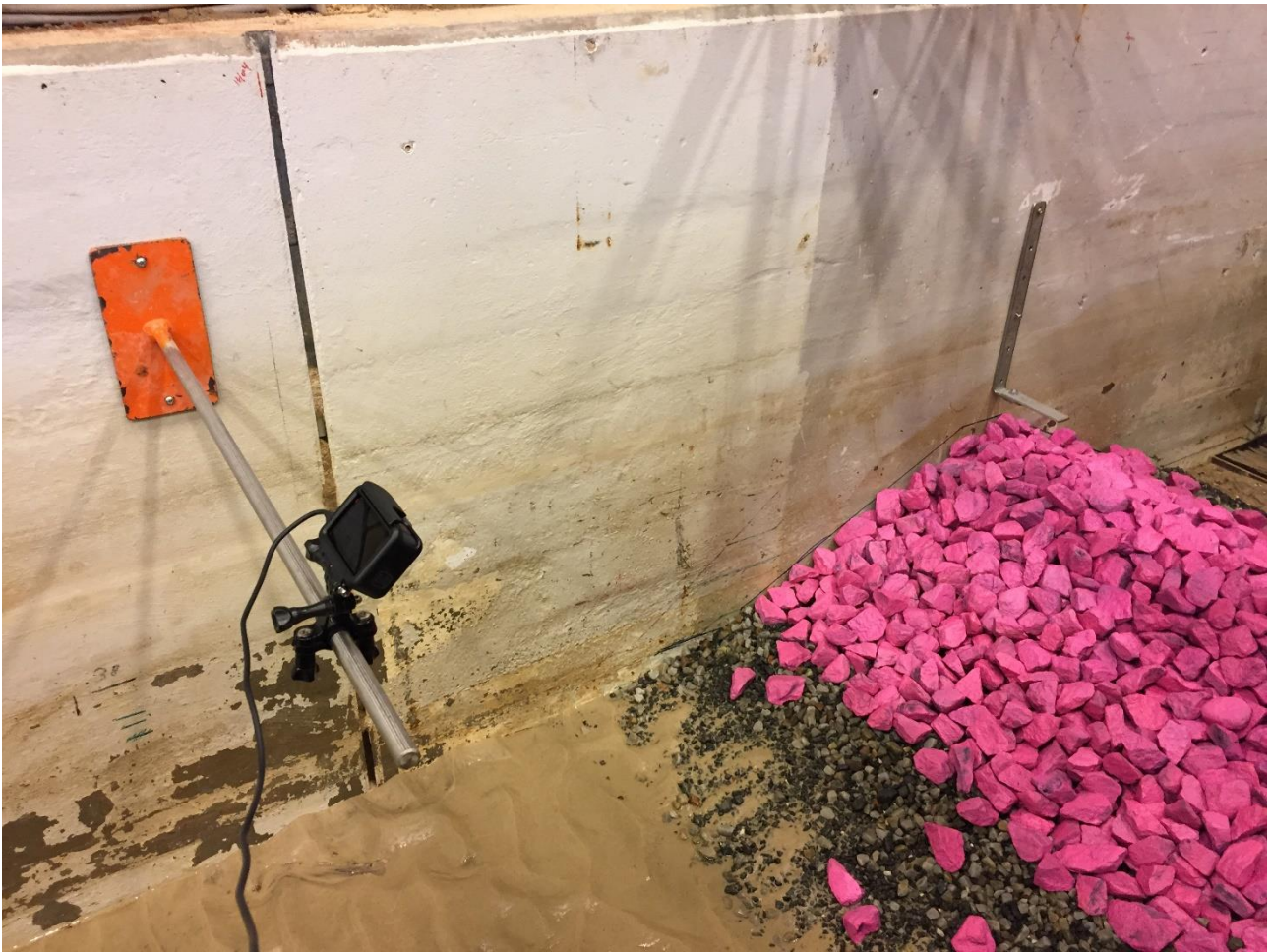
Figure 11: Camera in front of the breakwater, example with cross-section C1.
