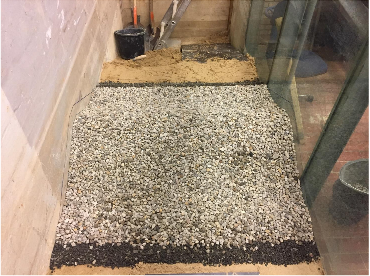
Figure 6: Breakwater with core and upper core for cross-section C1.
