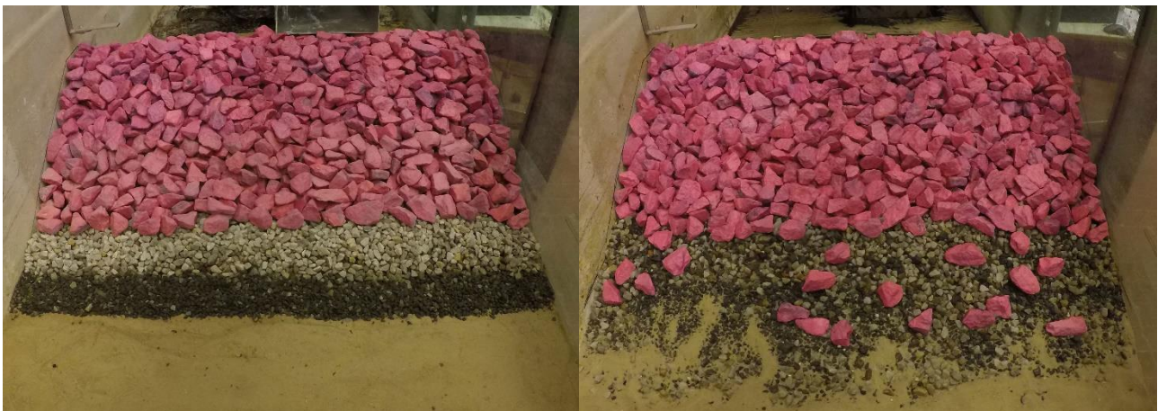
Figure 15: The front of the breakwater (C1) is shown on both pictures. Left shows before tests and right shows after Test 11.
