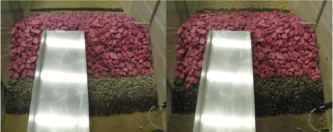
Figure 16: The rear of the breakwater (C1) is shown on both pictures. Left shows before test 1 and right shows after test 3.
