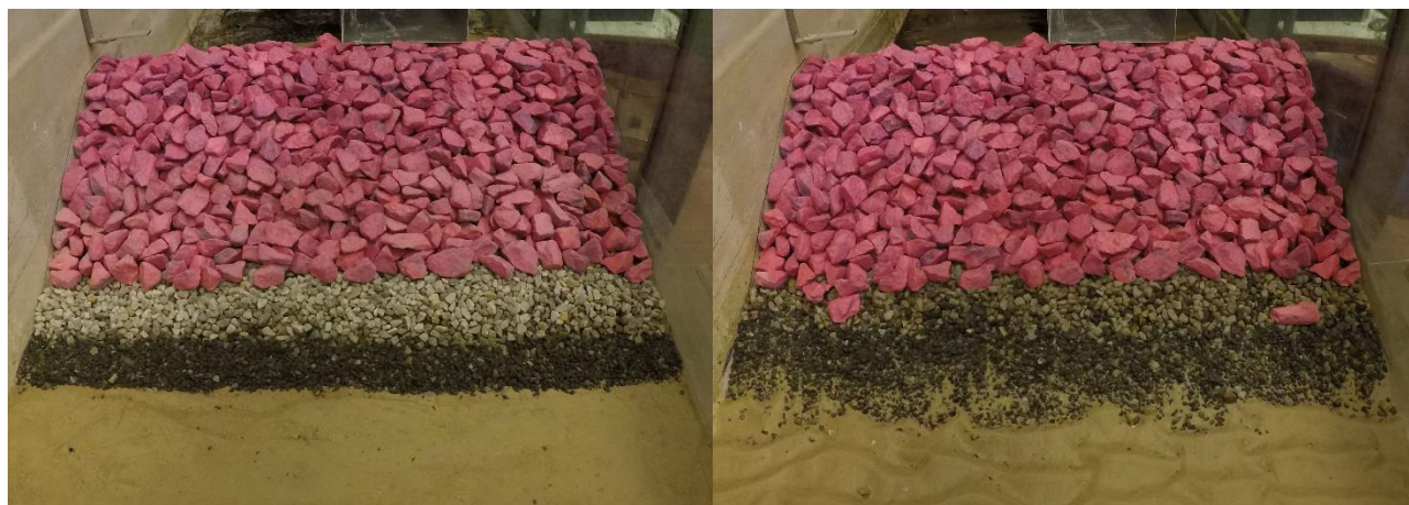
Figure 13: The front of the breakwater (C1) is shown on both pictures. Left shows before tests and right shows after Test 1.
