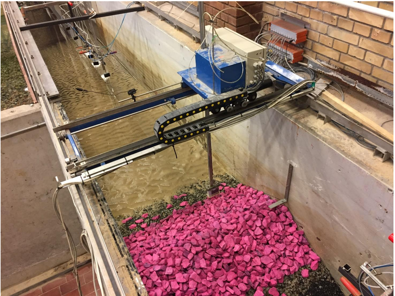
Figure 10: Profiler used to measure eroded area on the breakwater, example with cross-section C1.
