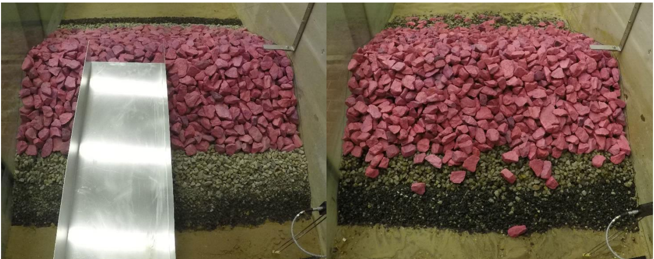
Figure 18: The rear of the breakwater (C1) is shown on both pictures. Left shows before Test 1 and right shows after Test 11.
