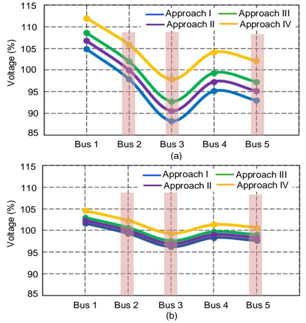
Fig. 3. Comparative numerical analysis of bus voltages with different control strategies – normalized by 400 V; (a) results of Case I with long feeders, (b) results of Case II with short feeders. **Approach I:** regulating average voltage of generator busses ( $V_1, V_4$ ), **Approach II:** regulating voltage of PCC ( $V_2$ ), **Approach III:** regulating average voltage of all busses, **Approach IV:** regulating average voltage of the weakest busses ( $V_3, V_5$ ).
