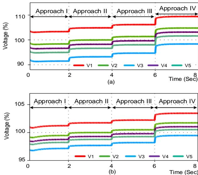
Fig. 5. Simulated normalized voltage of busses (based on 400 V): (a) considering long feeders (Case I), and (b) considering short feeders (Case II). Approach I: regulating average voltage of generator busses ( $V_1, V_2$ ), Approach II: regulating voltage of PCC ( $V_2$ ), Approach III: regulating average voltage of all busses, Approach IV: regulating average voltage of the weakest busses ( $V_3, V_5$ ).
