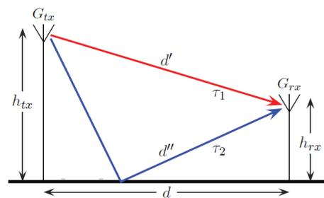
Fig. 1: Simplification with the 2 Ray model.
