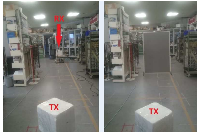
Fig. 6. Measurement scenario. Left in the figure the LOS case is shown and right in the figure the O-LOS case is shown. The biconical TX antenna, seen in the bottom of both scenarios, is encased in styrofoam as a part of its design.
