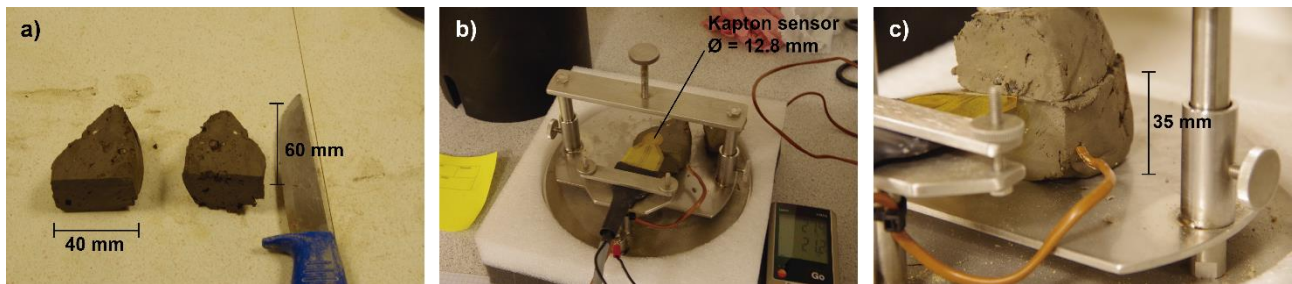
Figure 11: a) Halved moraine clay sample. b) Hot Disk kapton sensor ready to be placed between two specimens of soil. c) On-going Hot Disk testing, two-side measurement of a moraine clay sample (depth 8.5 m at Langmarsvej test site).
