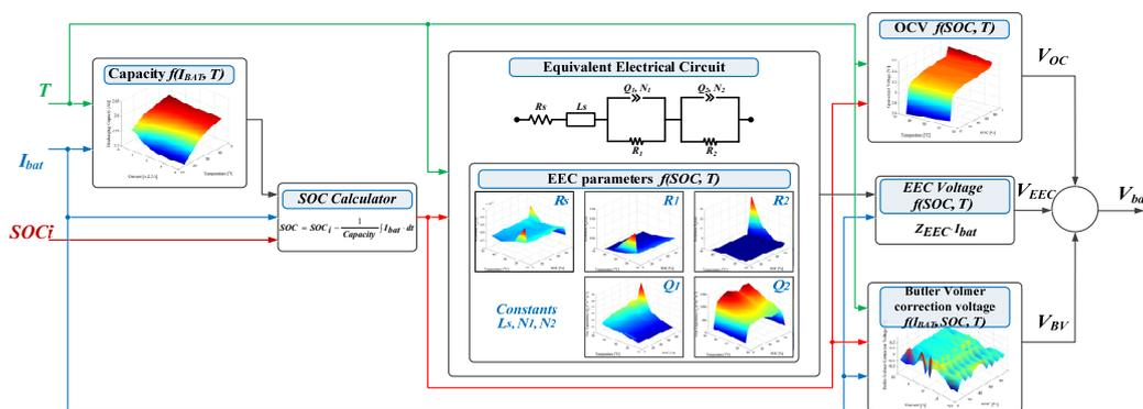
Figure 18. Block diagram implementation of the performance model for the LFP/C battery.
