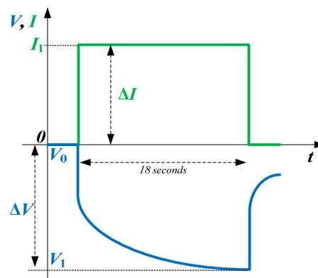
**Figure 7.** Theoretical voltage and current of Li-ion battery during impedance measurement with the current pulse technique.
