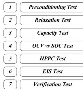
**Figure 2.** Test sequence for characterization of the LFP/C battery. OCV: open-circuit voltage; SOC: state-of-charge; and HPPC: hybrid pulse power characterization.
