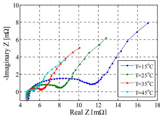
Figure 11. Dependence of the impedance spectra on the temperature; SOC = 50%.
