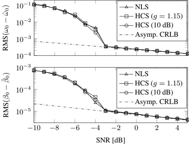
**Fig. 4.** Estimation accuracy as a function of the SNR. Settings:  $N = 250$ ,  $l = L = 6$ ,  $\omega_0 \sim \mathcal{U}(8\pi/N, 16\pi/N)$ ,  $\beta_0 \sim \mathcal{U}(-3/N^2, 3/N^2)$ ,  $A_i = 1$ ,  $i = 1, \dots, l$ , and  $\phi_i \sim \mathcal{U}(0, 2\pi)$ .
