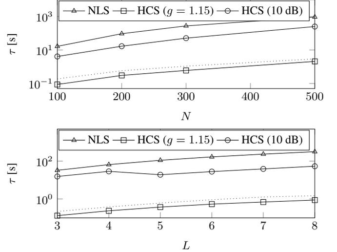
**Fig. 5.** The computation times for computing the objectives on the grid with  $F = 5NL$  and  $K = NL$ . Top:  $L = 6$  Bottom:  $N = 256$ . The dotted lines are the corresponding timing of the HCS ( $g = 1.15$ ) with the Nelder-Mead refinement step.
