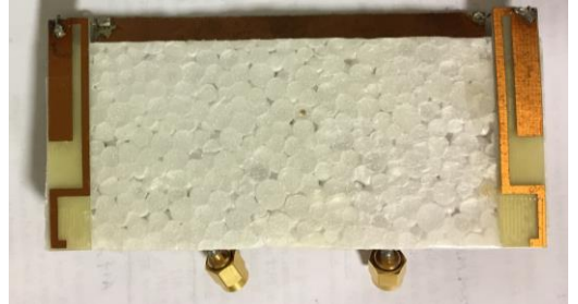
Fig. 3. Photo of the mockup handset antenna.
