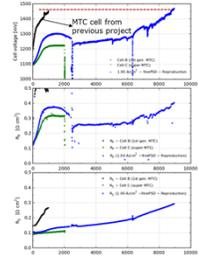
One-year SOEC single cell test under  $-1 \text{ A/cm}^2$  at  $800 \text{ }^\circ\text{C}$  conducted in the current project (blue curve).
