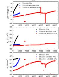
Long-term steam electrolysis durability tests under  $-1.25 \text{ A/cm}^2$  at  $800 \text{ }^\circ\text{C}$ . The cell degradation was reduced by a factor of 15, from  $714 \text{ mV}/1000\text{h}$  (black curve) to  $50 \text{ mV}/1000\text{h}$  (red curve).
