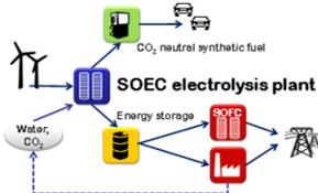
SOEC is a unique energy conversion technology that can provide regulating services to the electrical power grid by efficient storage of electrical energy as fuels. The fuels can be converted back to electricity by running the SOEC in the reverse power generation mode.
