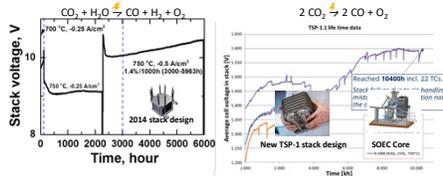
It has also been demonstrated that large SOEC stacks (TSP-1, 75 cell, rated power 7.5 kW) can be operated in a stable manner with a real world wind power production profile for grid balancing purpose.
