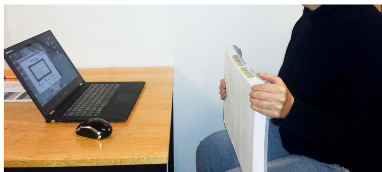
Fig. 1 Participant seated and squeezing the upper left corner of the Nintendo Wii Balance Board
