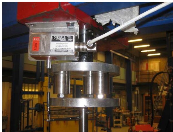
Figure 14: CPT displacement transducer
