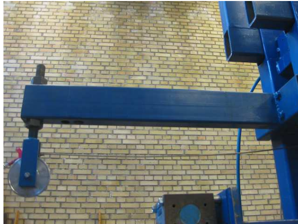
Figure 21: Cyclic loading frame
