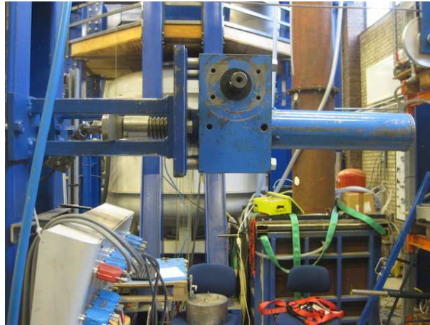
Figure 23: Static loading screw jack
