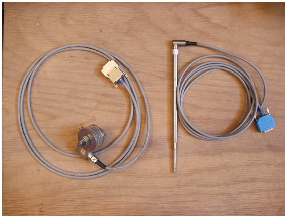
Figure 27: Force and displacement transducer
