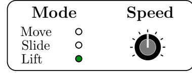
Fig. 3. Sketch of the utilized joystick, with three modes Move , Slide , and Lift , and a knob for adjusting the speed of the selected motion.
