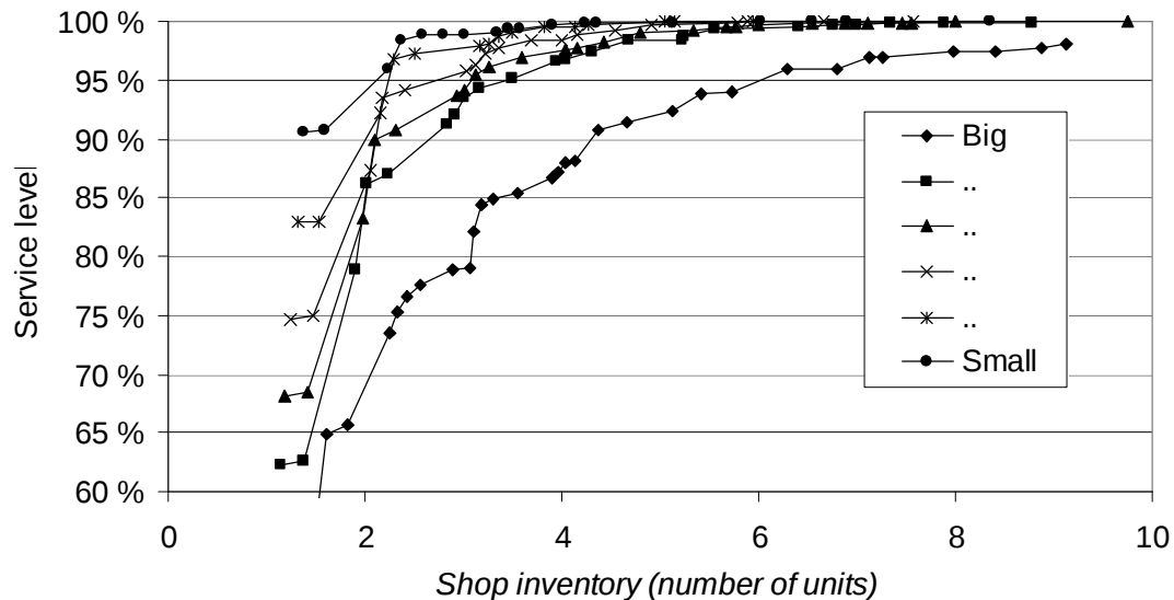
Figure 8: Service level versus inventory for different shop sizes in the manufacturing postponement concept (absolute number of units).
