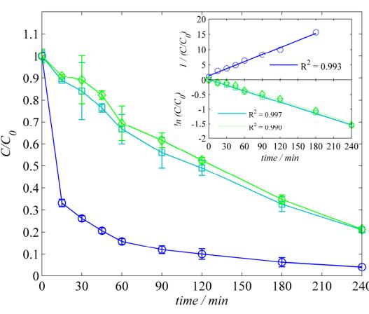
The evolution of the relative concentrations of  $(\circ)$  naphthalene,  $(\Box)$ fluoranthene, and (\dagger) pyrene during electrochemical oxidation in 0.10 M Na<sub>2</sub>SO<sub>4</sub> electrolyte at 200 mA cm<sup>-2</sup>. Subplot: The standard kinetic analysis, which showed difference in reaction kinetics.
