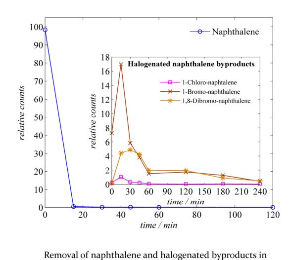
0.10 M NaCl + 0.001 M KBr (model sea water) at 25 mA cm<sup>-2</sup>
