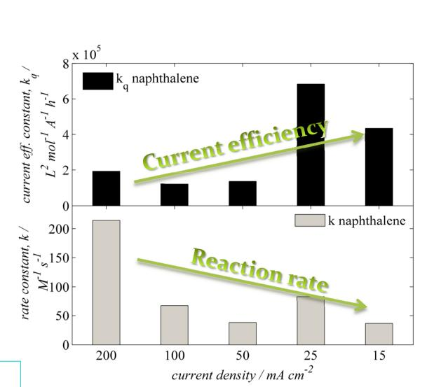
Comparison of reaction rates and current efficiencies at different current densities for naphthalene in 0.14 M NaCl electrolytes. Naphthalene is chosen as an example, but the trends were similar for all three PAHs.
