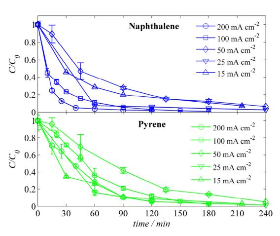
The influence of current density on the evolution in the relative concentrations during electrolysis in 0.14 M NaCl electrolyte.
