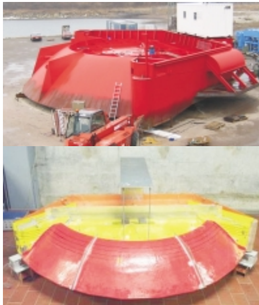
Figure 6: Photo showing the doubly curved ramp.
