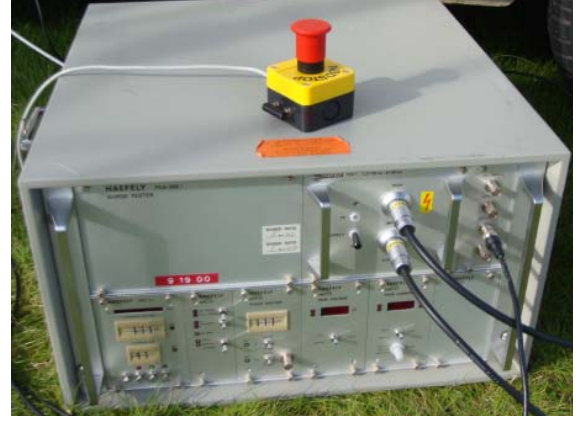
Fig. 8 A HAEFELY PC6-288.1 surge tester used to generate a 2 kV 1.2/50 μs impulse.
