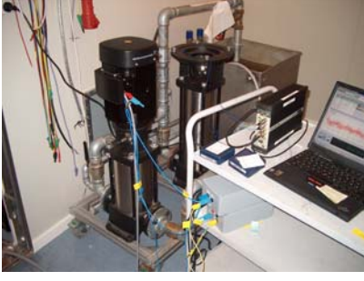
Fig. 3. The induction motor in a circulation system
