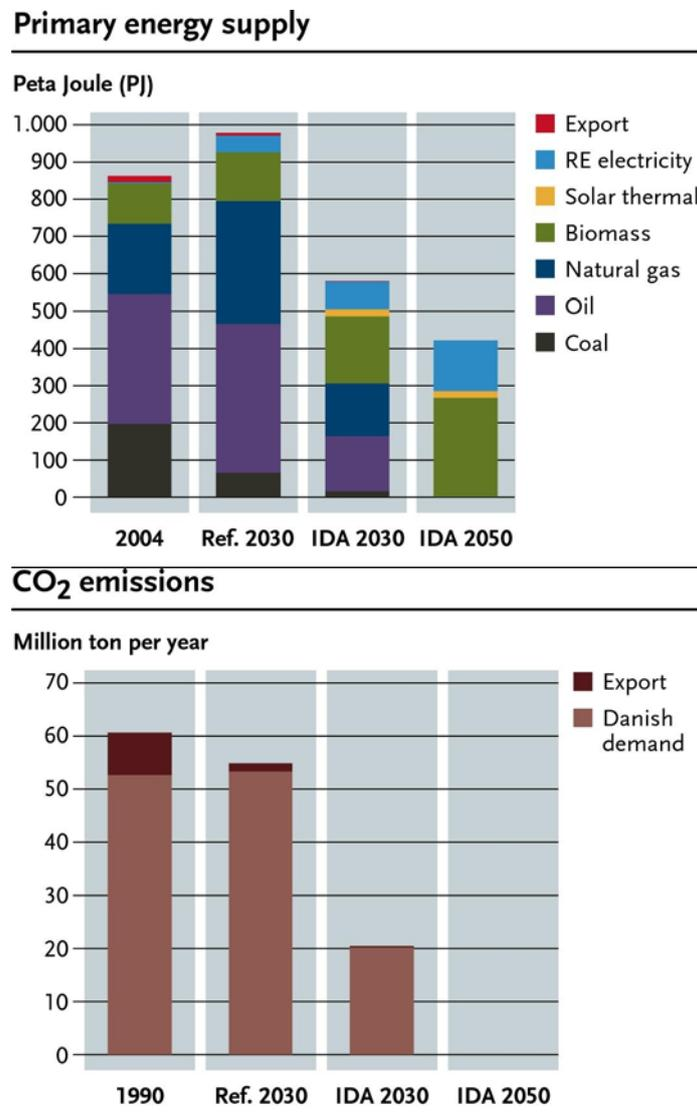
Figure 7. Primary energy supply and CO<sub>2</sub> emissions. CO<sub>2</sub> emissions are divided into domestic electricity demand and electricity net exports.
