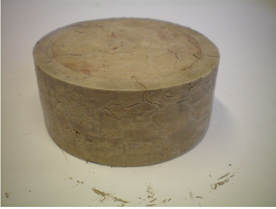
Figure 1: Fissured Søvind Marl after a consolidation test.
