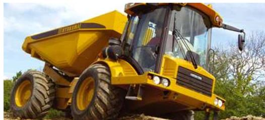
**Figure 1.** Hydrema 912DS Articulated Dump Truck.
