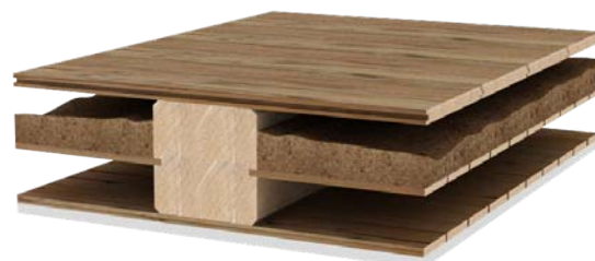
Existing floor construction in old housing: Typical Danish timber floor construction with pugging
