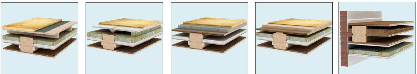
Examples of different solutions tested in the laboratory and/or in the apartment building, some fulfilling sound class C, some only class D
