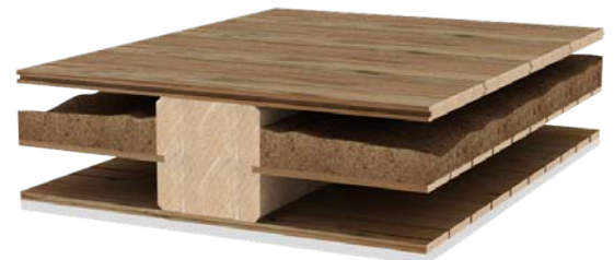
Existing floor construction in old housing: Typical Danish timber floor construction with pugging
