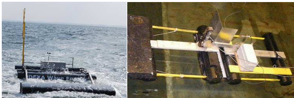
Figure 2: Model of DEXA deployed in Lymfjord (scale 1:10) and laboratory model (1:20 scale).
