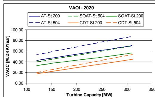
**Figures 5-6:** VAOI as a function of the turbine capacity for storage sized of 200,000m<sup>3</sup> and 504,000m<sup>3</sup> for the years 2010 and 2020.
