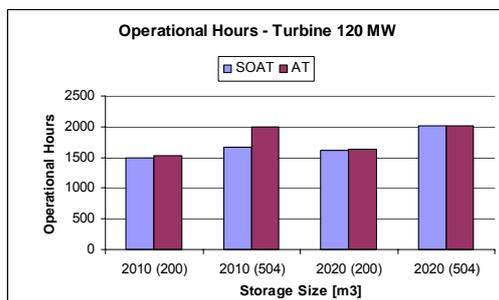
**Figure 7:** Number of turbine operational hours for a turbine capacity of 120 MW, storage sizes of 200,000m<sup>3</sup> and 504,000m<sup>3</sup>, and years 2010 and 2020.
