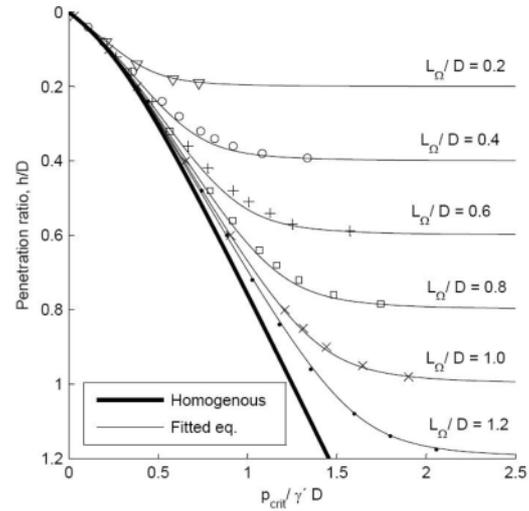
Figure 9. Normalized critical suction versus relative penetration. The critical suction is calculated with different ratios  $L_{\Omega}/D$ .
