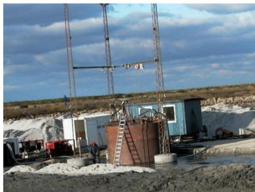
Figure 1. Installation tests on  $4 \times 4$  m buckets in a natural seabed at the test site in Frederikshavn, Denmark.
