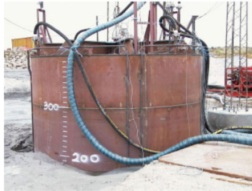
Figure 3. The critical suction has been achieved and soil failure by piping has occurred. The test was performed with a 4 \times 4 m bucket.
