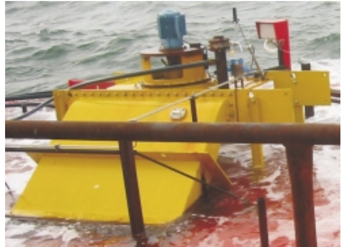
Figure 5: Kaplan turbine with Siphon inlet
