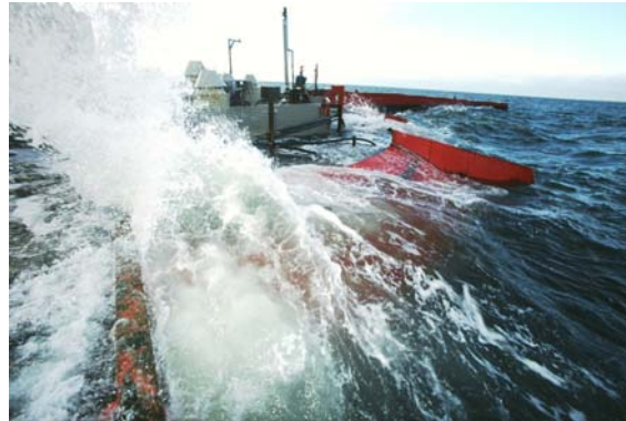
Figure 2: Good overtopping occurring on the Wave Dragon prototype in Nisum Bredning
