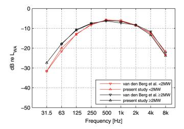
FIG. 15. (Color online) Normalized A-weighted apparent sound power levels in octave bands, means for two groups of turbines: < 2 and  $\ge 2$  MW and from two investigations: van den Berg *et al.* (Ref. 69), Appendix D and present investigation (converted to octave bands).
