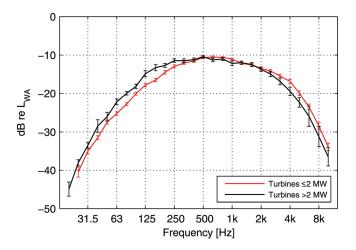
FIG. 4. (Color online) Normalized A-weighted apparent sound power levels in one-third-octave bands, means of two groups of turbines:  $\leq 2$  MW and > 2 MW. Error bars indicate  $\pm 1$  standard error of mean.
