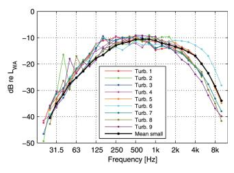
FIG. 5. Normalized A-weighted apparent sound power levels in one-third-octave bands, mean of 36 turbines  $\leq 2$  MW (bold line) and 9 individual turbines  $\geq 2$  MW
