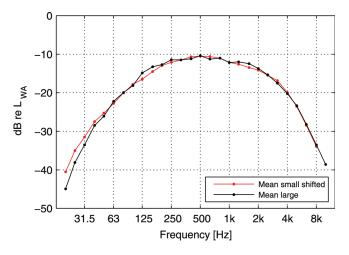
FIG. 17. (Color online) Normalized apparent sound power levels in one-third-octave bands. Mean of two groups of turbines:  $\leq 2$  and > 2 MW, group of turbines  $\leq 2$  MW shifted one third of an octave down in frequency. (Turbine 6 disregarded above 2 kHz, see Sec. III A 2.)
