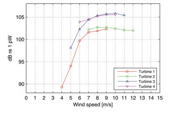
FIG. 8. (Color online) A-weighted apparent sound power level,  $L_{\rm WA}$ , as a function of wind speed for turbines 1–4 (turbine color code as in Fig. 5).
