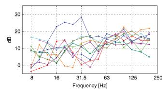
FIG. 10. Sound insulation measured for ten rooms.
