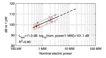
FIG. 13. (Color online) Apparent sound power level ( $L_{\rm WA}$ ) as a function of turbine size, four turbines below 450 kW excluded, wind speed 8 m/s. Linear regression line, standard error of estimates (s.e.e.) 1.64 dB. Extrapolation dashed, 90 % confidence intervals (dotted) based on s.e.e.
