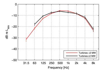
FIG. 14. (Color online) Normalized A-weighted apparent sound power levels in octave bands, means for two groups of turbines: <2 and  $\geq 2$  MW. Data from van den Berg et al., <sup>69</sup> Appendix D. Error bars indicate  $\pm 1$  standard error of mean. (None of the large turbines was measured in the 31.5-Hz octave band).
