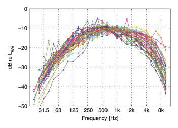
FIG. 3. Normalized A-weighted apparent sound power levels in one-third-octave bands. Forty-five turbines with nominal electric power 75 kW–3.6 MW. (Normalized meaning that  $L_{\rm WA}$  for the individual turbine has been subtracted from all one-third-octave-band levels.)
