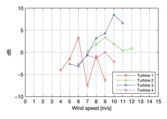
FIG. 6. (Color online) Tonal audibility,  $\Delta L_{\rm ta}$ , as a function of wind speed for turbines 1–4, reference direction (turbine color code as in Fig. 5).
