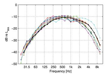
FIG. 16. Normalized A-weighted apparent sound power levels in one-third-octave bands, individual turbines > 2 MW and mean of 36 turbines  $\le 2$  MW. Peaks in one-third-octave bands below 200 Hz have been removed from the large turbines by replacing the levels at the peaks by levels obtained by linear interpolation between the levels at the two adjacent one-third-octave-band frequencies (turbine color code as in Fig. 5).
