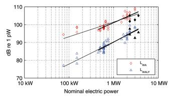
FIG. 1. (Color online) Apparent sound power levels ( $L_{\rm WA}$  and  $L_{\rm WALF}$ ) in the reference direction as a function of turbine size. Wind speed is 8 m/s. Regression lines: all turbines included (thin lines), four turbines below 450 kW excluded (bold lines). Black-filled marks are for turbines 1–4.
