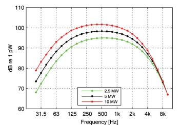
FIG. 19. (Color online) Estimated A-weighted sound power levels in one-third-octave bands for turbines around 2.5, 5, and 10 MW. Values and assumptions are taken from Table III.
