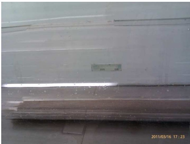
Figure 9, Initial conditions and creation of the sediment dunes inside the pipe ( D = 240 mm). Water flow velocity V = 0.4 m/s
