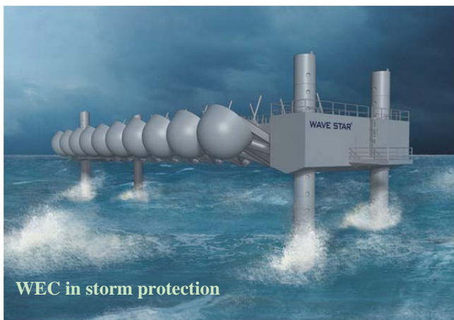
Fig. 5 Artist impression of a commercial Wave Star WEC
