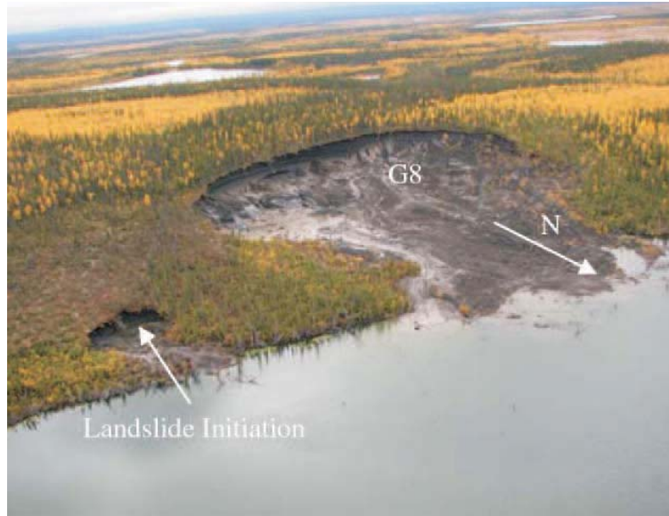
Figure 1.5 Example of a thaw induced slide, Mackenzie Valley, Canada. The area of the largest slide shown is about 30,000m 2 . Reproduced with permission from the work of Wang et al. (2009).
