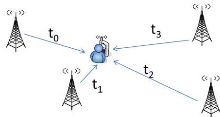
Fig. 2. Message flow in device-based conventional positioning.
