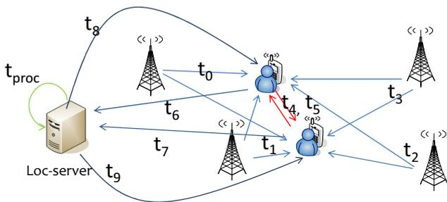
Fig. 3. Message flow in centralized cooperative positioning.
