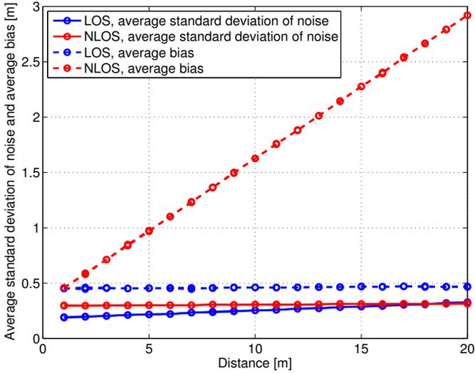
Fig. 7. Average ranging error model parameters vs. distance
