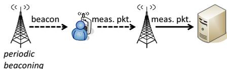
Fig. 4. Message flow for beacon measurements in cooperative localization.
